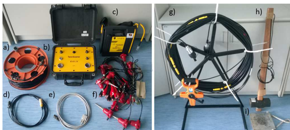
Figure 1: a) Extension of the trigger, b) RAS-24, c) 12v battery, d) Trigger e) Serial cable, f) 12 geophones, g) Connection cable of 120m geophones, h) 8kg hammer and, i) Aluminum plate 20x20 cm.
