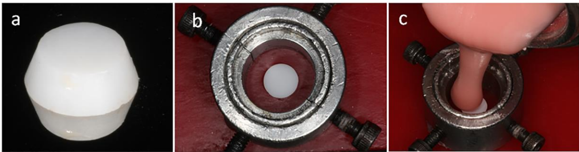
Figure 1: a) zirconia sample; b) metal matrix positioned on the wax and the sample centralized in the matrix; c) the matrix filled with self-cured acrylic resin.
