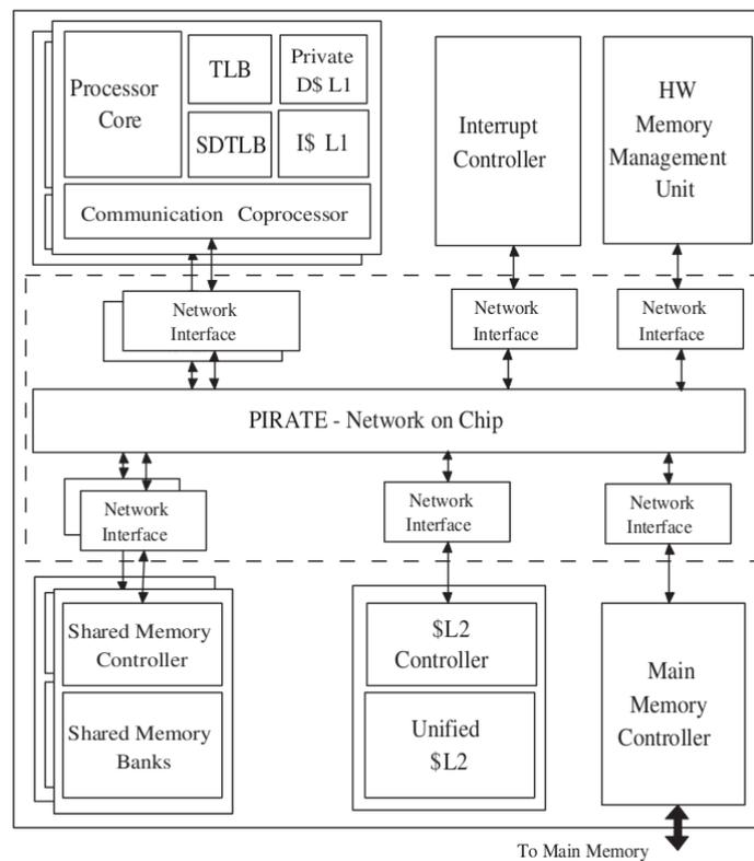
Figure 4 – Multiprocessor architecture proposed by [MON06].
