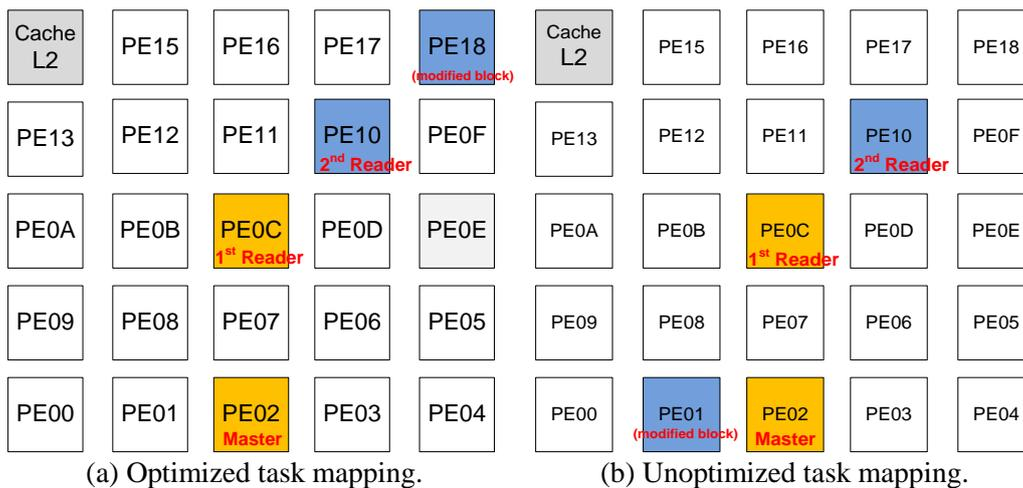
Figure 48 –Task mappings for the T state optimization.
