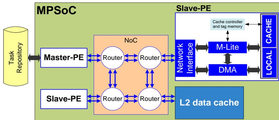
Figure 17 - MPSoC with a two level memory hierarchy – shared memory and caches (only Slave-PEs may contain caches).
