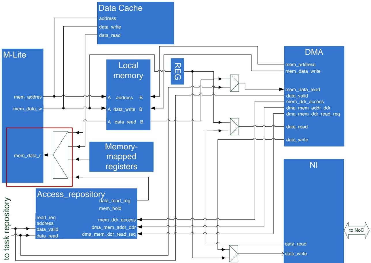
Figure 18 - Internal modules of the PLASMA processor.
