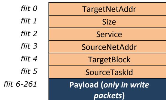
Figure 20 - Packet format for shared memory operations.
