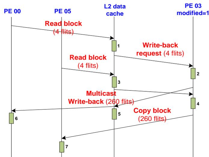
Figure 28 - Sequence diagram for the T state.
