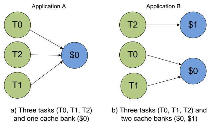
Figure 42 – Two different implementation of a MM application using 3 tasks.
