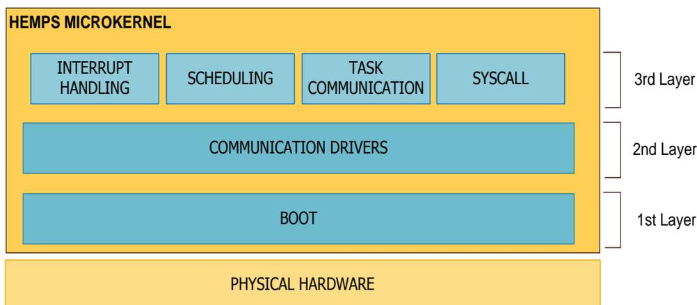
Figure 13 - HeMPS Microkernel Layers.
