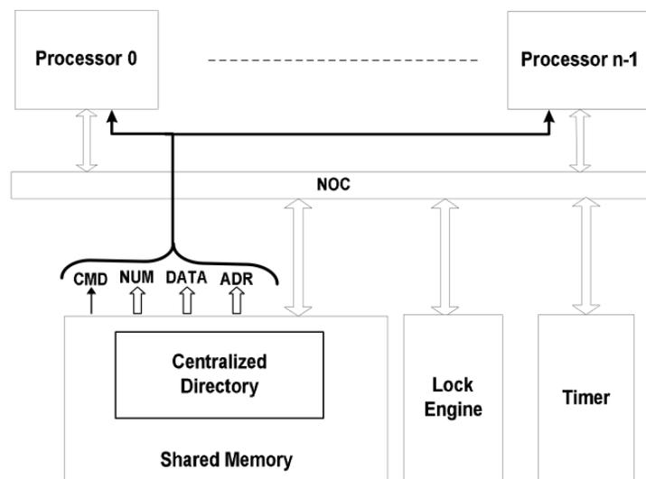
Figure 7 – NoC-based MPSoC architecture with an exclusive bus for cache coherence transactions [CHT09].
