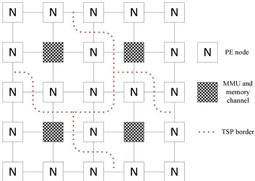
Figure 3 – NoC view of TSP partitions and positioning of MMU and PE nodes.
