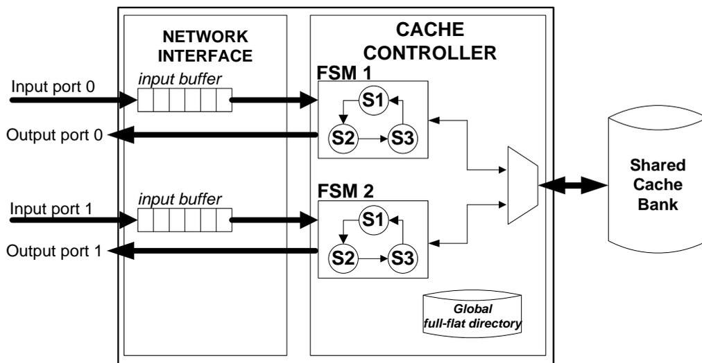
Figure 19 – Internal architecture of the L2 cache module.
