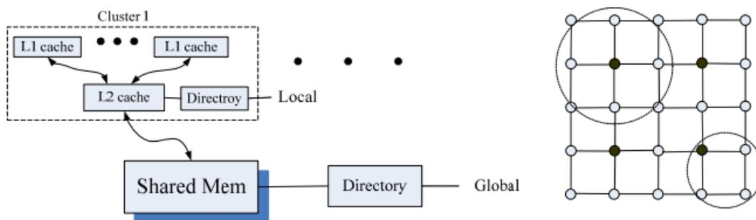
Figure 5 – In the left, it is shown the architecture of the HEAD node. In the right, each circle comprises a cluster region [YUA08].
