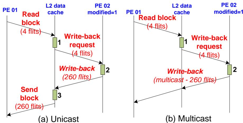
Figure 25 - Sequence diagram for a read operation of a modified cache block.
