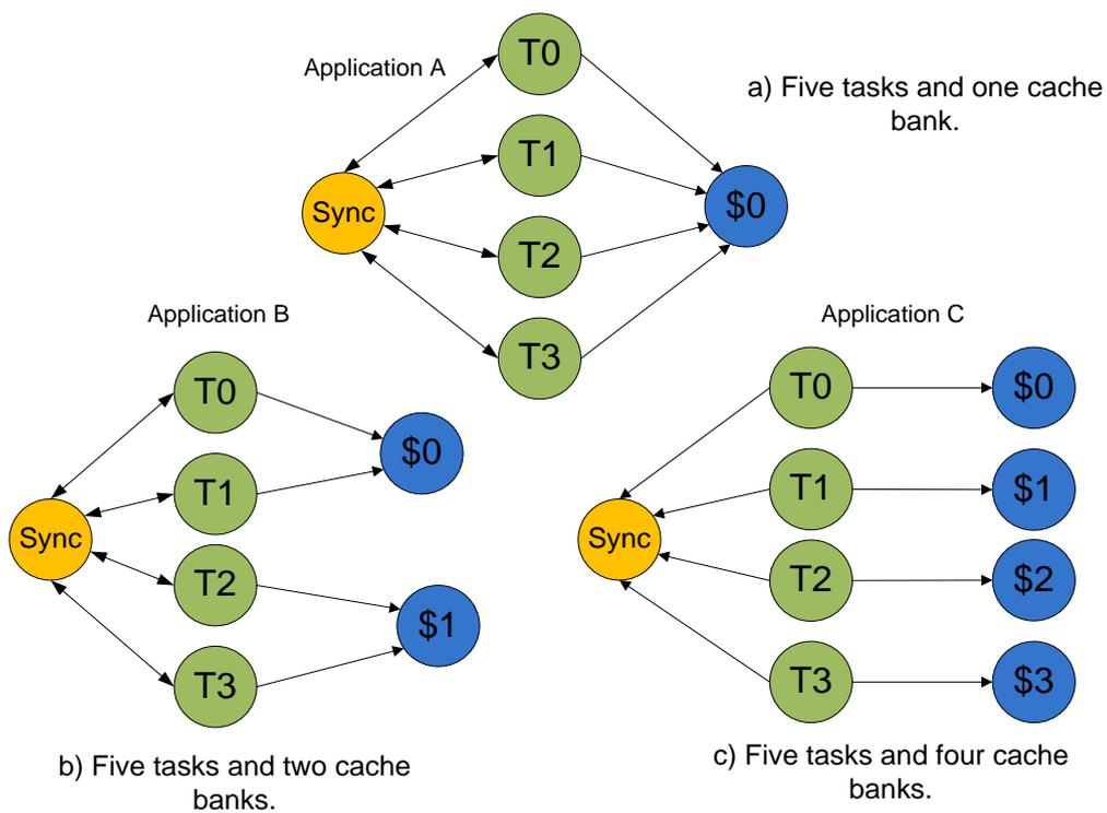
Figure 43 – Tasks graphs for equation solver application.
