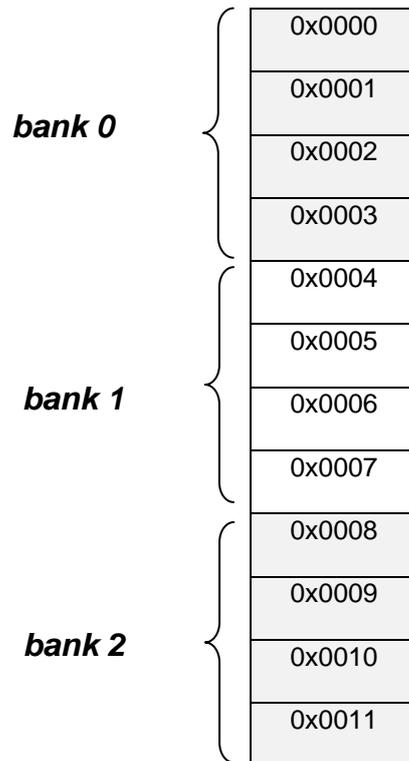
Figure 22 – Example of address space division in cache banks, assuming four blocks per L2 cache bank.
