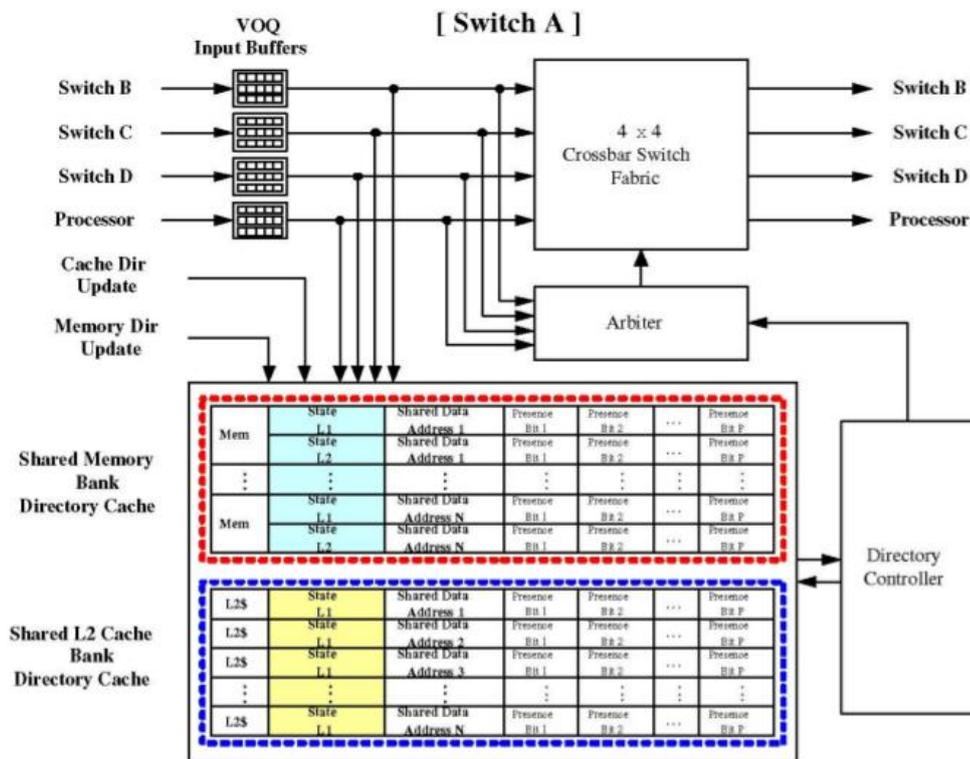
Figure 1 – DCOS switch architecture proposed by [KIM06].
