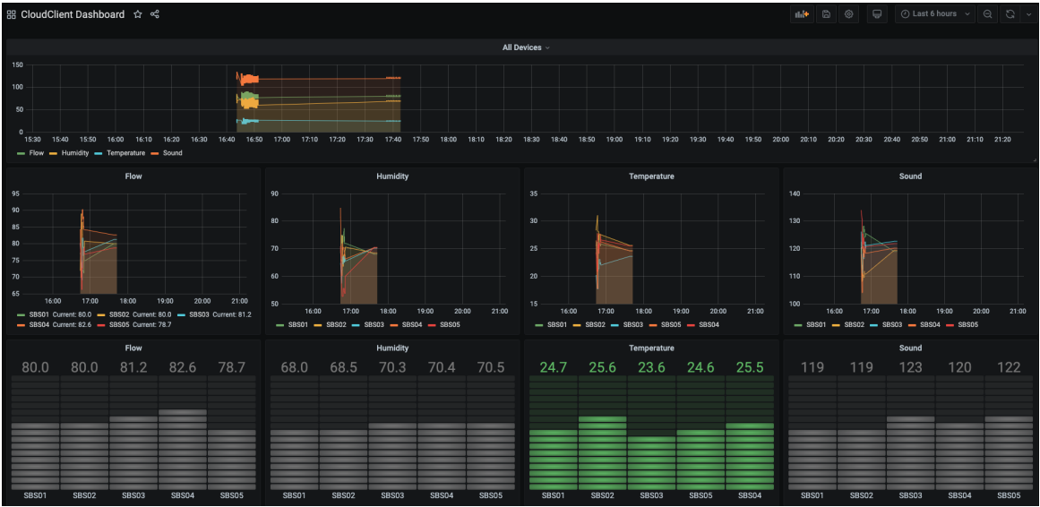
Figure 5.7 – Readings collected from Grafana. The monitoring layer in this scenario is built over the data stored in the Cloud Database. The readings refer to Flow, Humidity, Temperature, and Sound considering five different sensors SBS01, SBS02, SBS03, SBS04, and SBS05.
