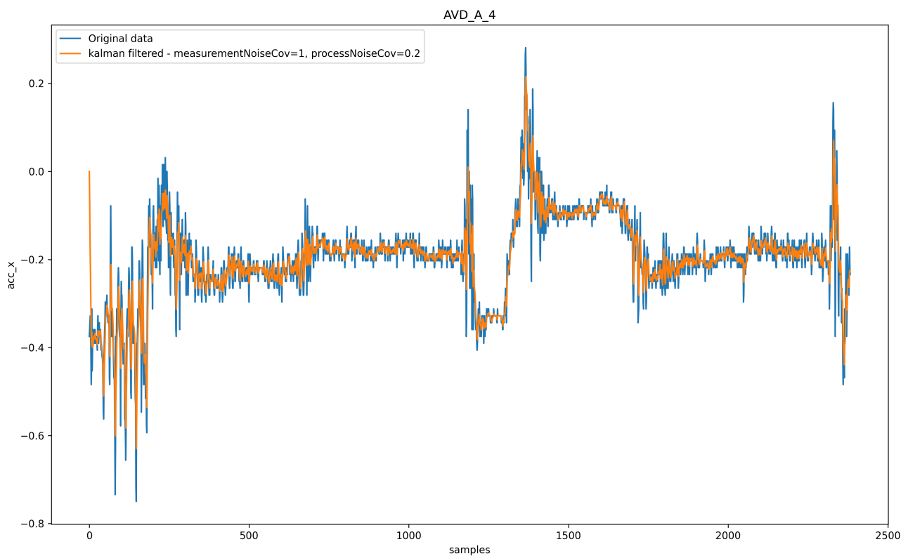
Figure 4.8 – Original sensor data and finished Kalman filtered data (Source: Author).
