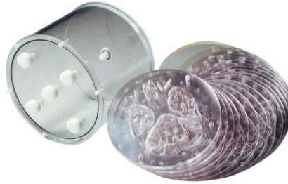
Figure 1. Hoffman 3D brain phantom consists of a cylinder with 40 independent cross-sections. Source: BIODIX (2021).
