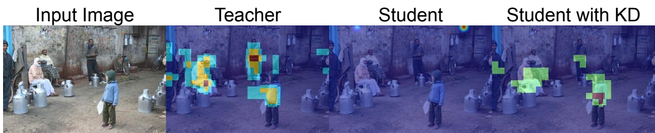
Figure 5.8 – Learned features visualization with Grad-CAM, from YOLOv3, YOLOv3-Mobile in default training, and YOLOv3-Mobile with KD fts 36, 91. Image generated using the second YOLO Head and the first anchor box.
