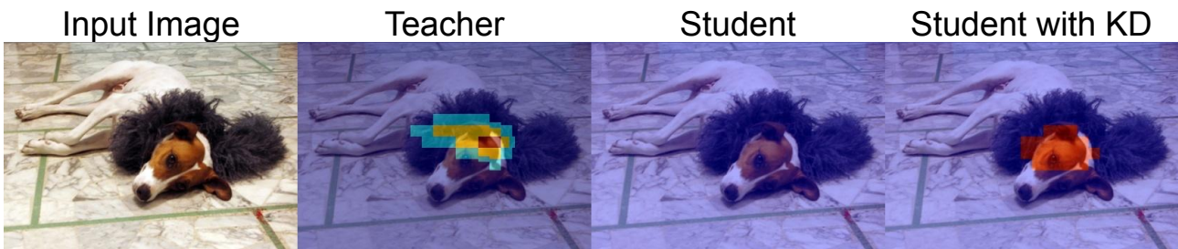
Figure 5.12 – Learned features visualization with Grad-CAM for YOLOv3, YOLOv3-Mobile with default training, and YOLOv3-Mobile with KD GAN. Image generated using the second YOLO Head and the third anchor box.
