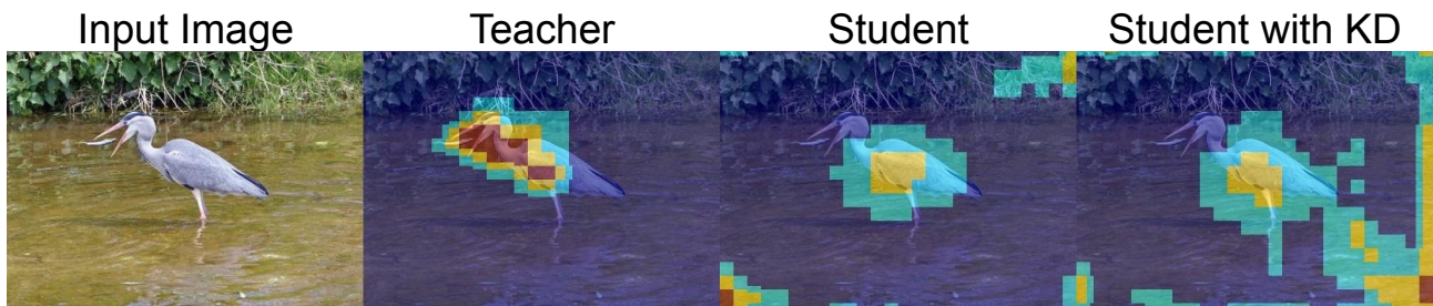
Figure 5.1 – Learned features visualization with Grad-CAM for YOLOv3, YOLO Nano with default training, and YOLO Nano with KD GAN. Image generated using the second YOLO Head and the first anchor box.
