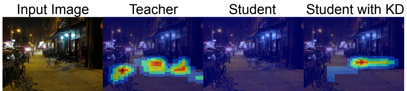
Figure 5.23 – Learned features visualization with Grad-CAM for YOLOv3, YOLOv3-Mobile with default training, and YOLOv3-Mobile with KD fts 91. Image generated using the first YOLO Head and the first anchor box.
