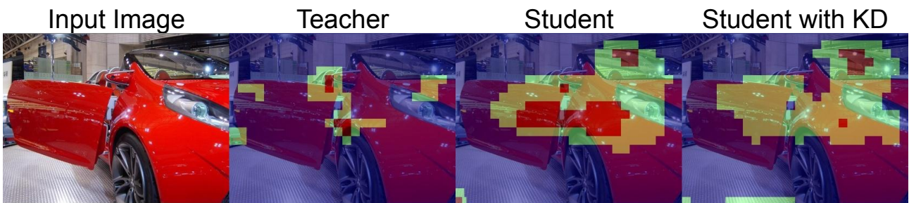
Figure 5.5 – Learned features visualization with Grad-CAM for YOLOv3, YOLO Nano with default training, and YOLO Nano with KD fts 79. Image generated using the second YOLO Head and the first anchor box.
