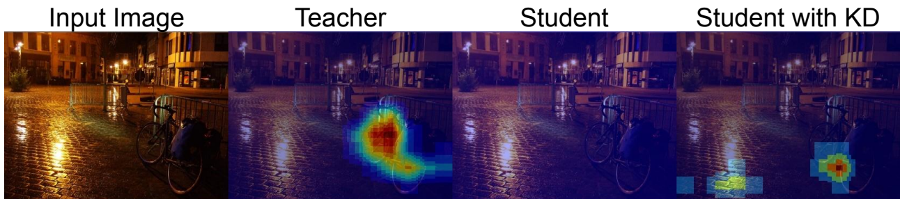
Figure 5.21 – Learned features visualization with Grad-CAM for YOLOv3, YOLOv3-Mobile with default training, and YOLOv3-Mobile with KD fts 36, 91. Image generated using the first YOLO Head and the third anchor box.
