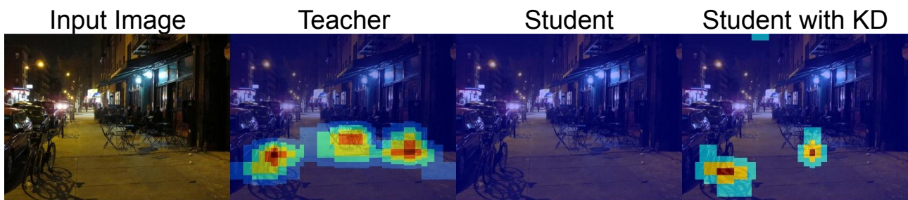
Figure 5.25 – Learned features visualization with Grad-CAM for YOLOv3, YOLOv3-Mobile with default training, and YOLOv3-Mobile with KD GAN. Image generated using the first YOLO Head and the third anchor box.
