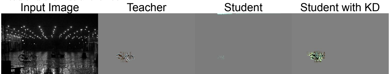
Figure 5.19 – Learned features visualization with Grad-CAM for YOLOv3, YOLO Nano with default training, and YOLO Nano with KD fts 79. Image generated using the second YOLO Head and the first anchor box.
