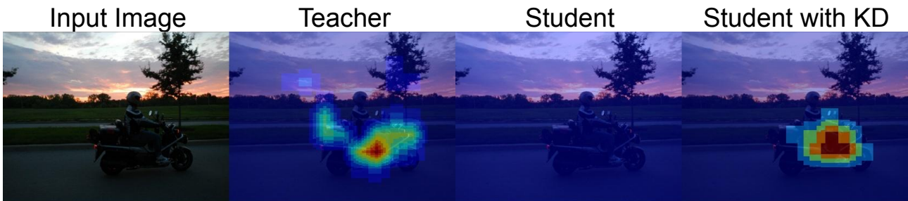
Figure 5.24 – Learned features visualization with Grad-CAM for YOLOv3, YOLOv3-Mobile with default training, and YOLOv3-Mobile with KD fts 91. Image generated using the first YOLO Head and the first anchor box.
