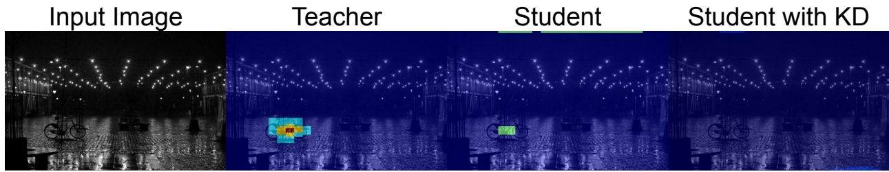
Figure 5.14 – Learned features visualization with Grad-CAM for YOLOv3, YOLO Nano with default training, and YOLO Nano with KD GAN. Image generated using the second YOLO Head and the first anchor box.
