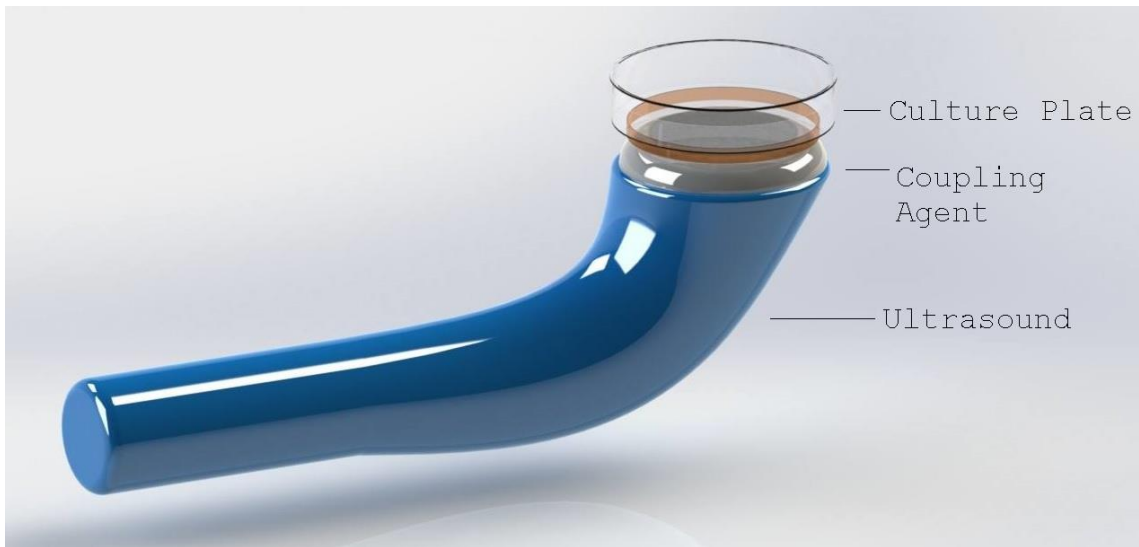
Figure 1: Schematic representation of ultrasound exposure system on the cell culture plate.
